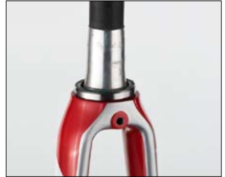
Figure 6. Lower bearing on fork crown
